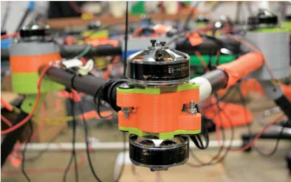
LEFT: One of the motors on the heavy-lift drone platform developed for Duke's entry in the Shell Ocean Discovery XPRIZE Competition
