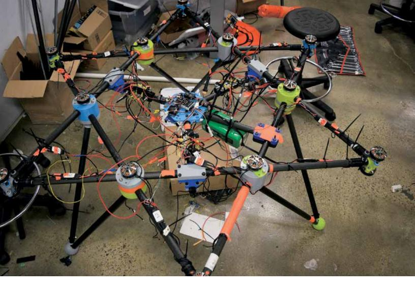
Top view of the heavylift drone platform developed for Duke's entry in the Shell Ocean Discovery XPRIZE Competition. Even students with minimal piloting experience are able to fly small-scale drones there with the protection of safety nets.
