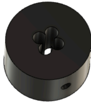
Figure 6: CAD Model for 2x2 Array Holder
